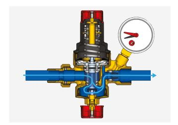
The water duct fluid enters the R150M filling unit and loads it up to the required pressure (calibration pressure).
