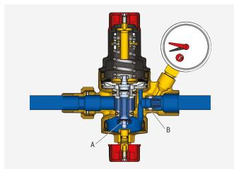
When the system reaches the desired pressure, the stopper (A) closes without letting in any fluid.
