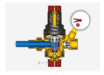
The R150M filling unit automatically reintegrates the installation water when the pressure drops below the calibration value, up to restoring the desired pressure.
