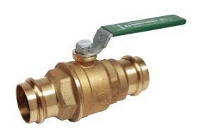
Ball valve, with press connections (for copper pipe complying with EN 1057; for stainless steel pipe complying with EN 10217-7 and EN 10312; for carbon steel pipe complying with EN 10305-3), specific for domestic water. Full port.
