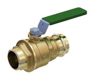
Ball valve, with male threaded-press connections (for copper pipe complying with EN 1057; for stainless steel pipe complying with EN 10217-7 and EN 10312; for carbon steel pipe complying with EN 10305-3), specific for domestic water.
